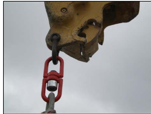
Figure 2. – Swivel allows unrestricted rotation but reduces available headroom
