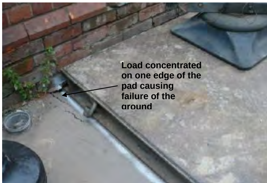
Figure D3 - Example of the Effect of an Offset Outrigger on a Pad
