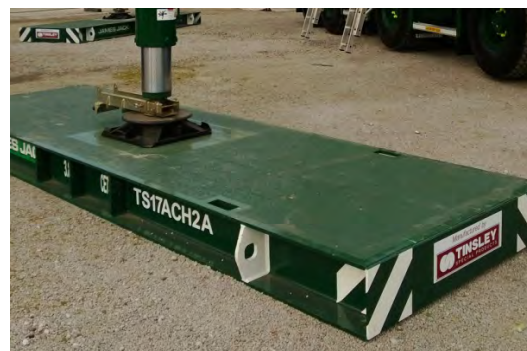
Steel Pad in Use
